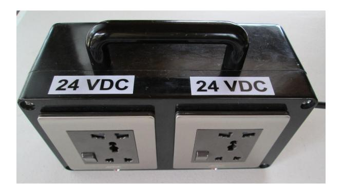
2 x 24VDC power supply with 2 port plug in 24VDC flood light option
